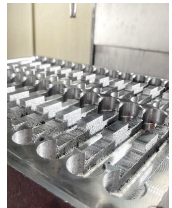
Interrupted Pocket milling operation
