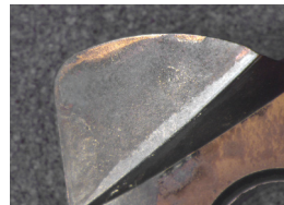
Flank and Rake wear after 45 min
