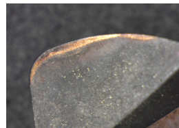
Flank and Rake wear after 67 min
